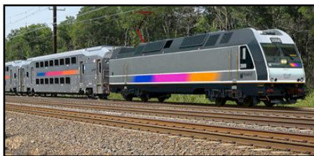
Bombardier Dual-Mode Electric and Diesel Locomotive Ordered by NJT and Montreal's AMT
